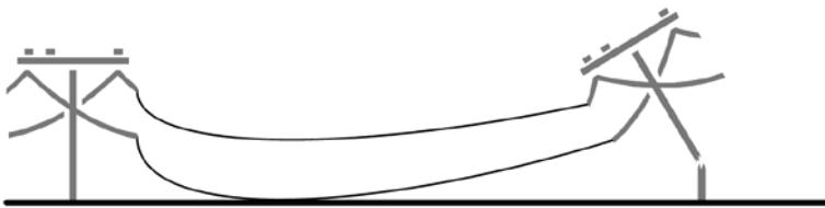
Figure 1: Downed Conductor
