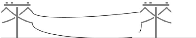
Figure 2: Downed Broken Conductor
