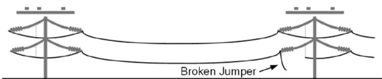
Figure 3: Broken Conductor That Is Not Downed
